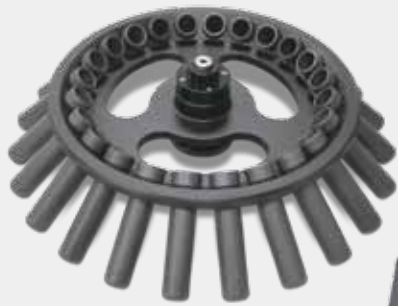
Sleeve, GLB-15A-FA 4,000 rpm / 3,134 xg
