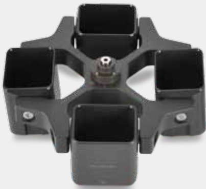
Bucket, GLB-r250-r250 4,000 rpm / 3,134 xg
